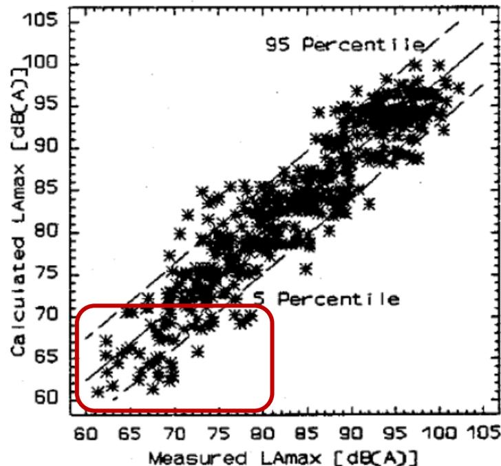
Wendover HS2 had observed that in the highlighted area (below 71dB calculated), the observed figures appeared to be higher than calculated. This is the range which affects almost all receptors in Wendover which are above night-time  $L_{Amax}$  LOAEL. The data represented by the points on this chart within the red box were extracted to a table (see Appendix A). There were 48 data points which provides a sufficiently large sample for this analysis.
