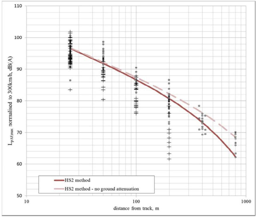
The rectangles represent downwind conditions and the crosses upwind conditions. The lower line represents the HS2 model, which is valid for downwind conditions. It will be seen that for the lowest group of points (800m), in the range up to 70dB, the measured results are consistently above the calculated results and the average difference is 2.5dB. This set of data would therefore confirm the finding from the AEL Paper that there is a consistent error of around this magnitude.
