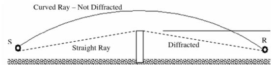
When the barrier is close to the track, the effect is small and it is likely that the HS2 noise model accounts for this, as it is validated for a variety of noise barriers including cuttings and bunds. However when the barrier becomes more distant from the line, the effect becomes significant. This particularly applies when natural landform is treated as a barrier. It is unlikely the HS2 model was validated for this situation.
